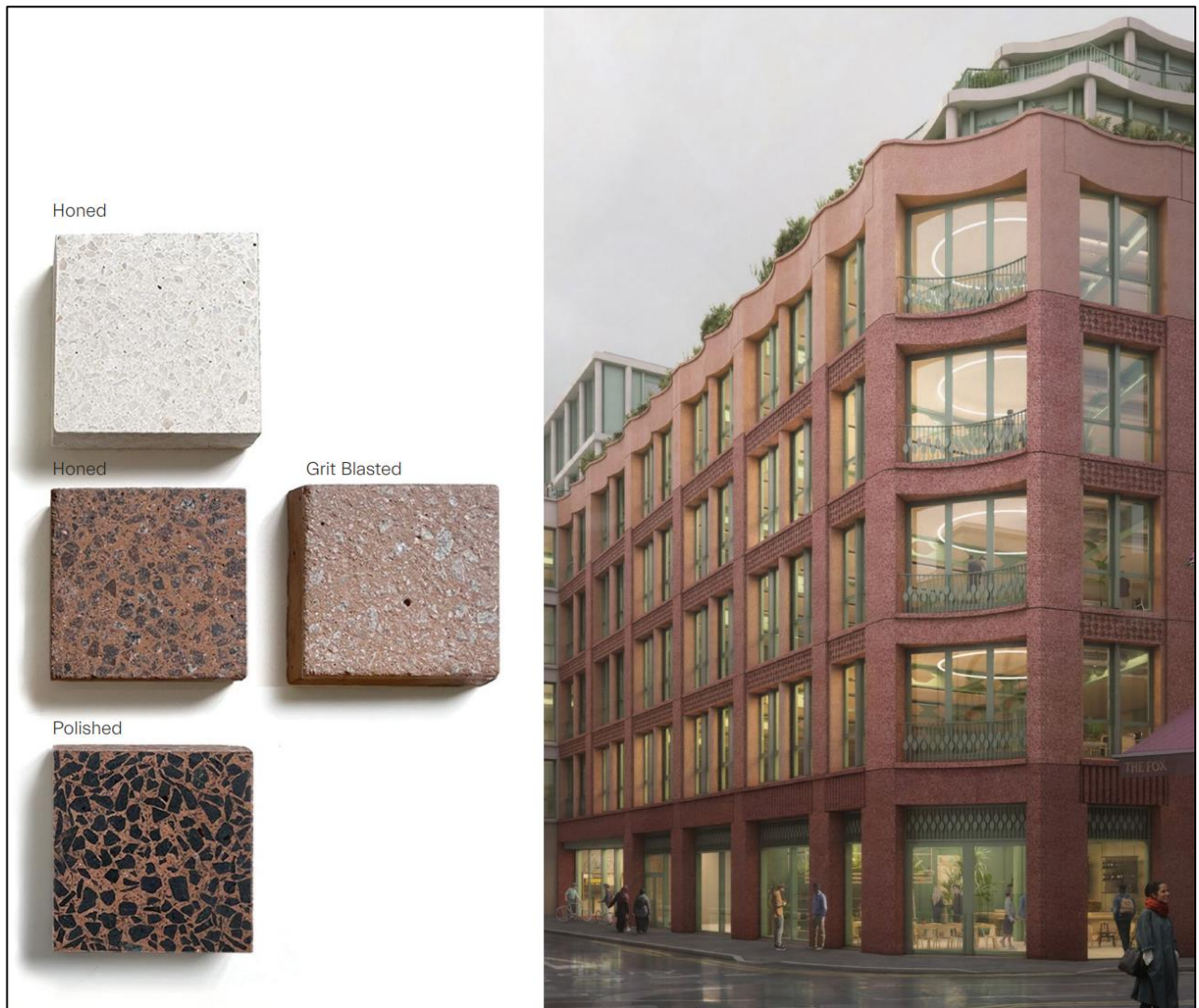
Figure 25: Material Palette of the 'Showroom' element to Paul Street and the eastern sides of Epworth Street and Clere Street
